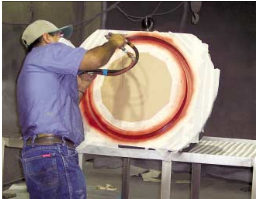
Spray booth operations resulted in evaporation of VOCs from metal parts, but destruction is not achieved without the addition of specific technology (photo by J. Weiler).
